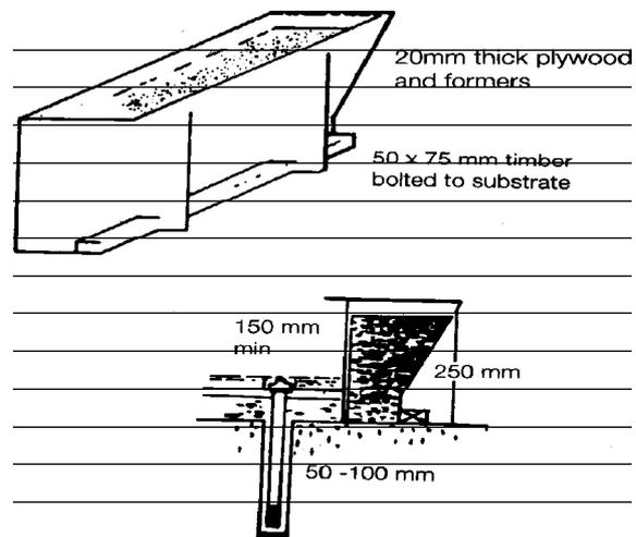
Pouring should be from one side of the void to eliminate any air or presoaked water becoming trapped under the base plate. It is advisable to pour the grout across the shortest distance of travel. The grout head must be maintained at all times so that a continuous grout front is achieved.
